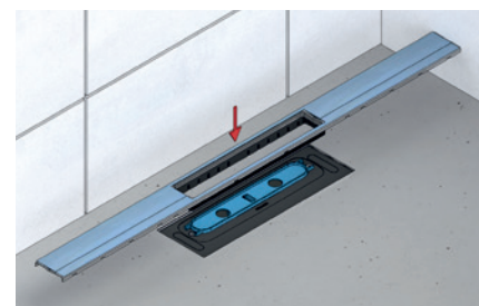
3. Insert the shower channel into the adhesive (like a tile)
